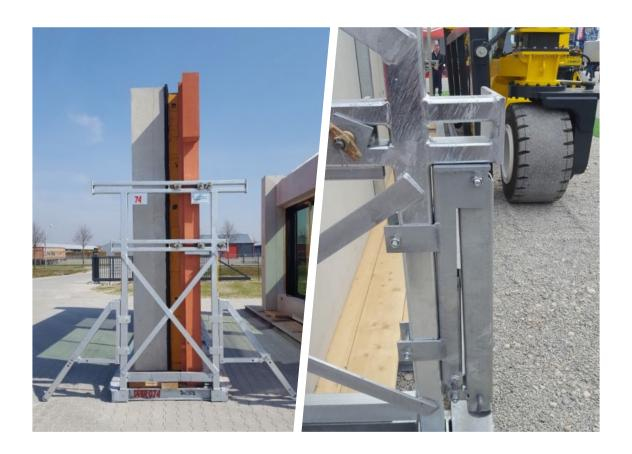
Blue Workx has developed a forklift pick-up yoke for secure and damage-free transport of empty inside loader pallets. With this yoke a 8 tonnes or heavier forklift truck can be used to position an empty pallet in the production hall without causing any damage.
