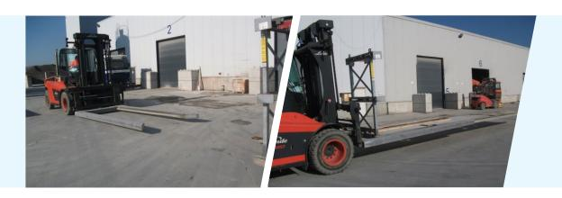
For the woodworking industry, Blue Workx has developed an inside loader pallet for transporting prefab wooden walls. Smart placement of the posts offers maximum width of the loading platform, creating space to transport more units.
