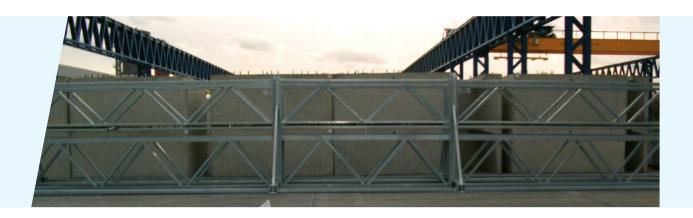
A walkway has been created along the length of the storage frame. This provides a safe and ergonomic area from where employees can carry out work, such as placing and securing units.
