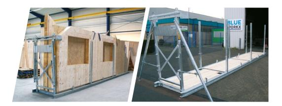
Part of our range are pallets with a solid steel floor. With these pallets transporting walls with a height of 4.25 meter is no problem. Adding a clearance of 13 cm, the total transport height is 4.40 meter, and a one-time permit will suffice for transport to almost any construction site.
