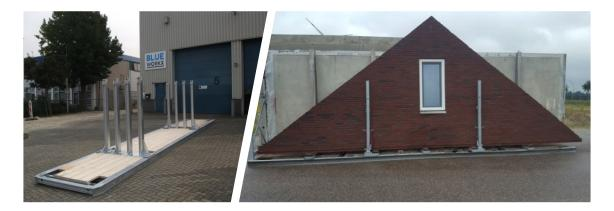
For the transport of special units, fittings can be mounted to the standard clamping posts of the inside loader pallets. A clamping system is used for quick and rock-solid attachment of the fittings to the pallet floor.
