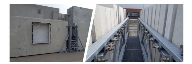
We can also offer simple pin frame storage frames, based on a design that has been in use by the concrete industry for many years.
